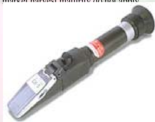
Fig 3. Hand-held refractometer for determining fruits maturity.
